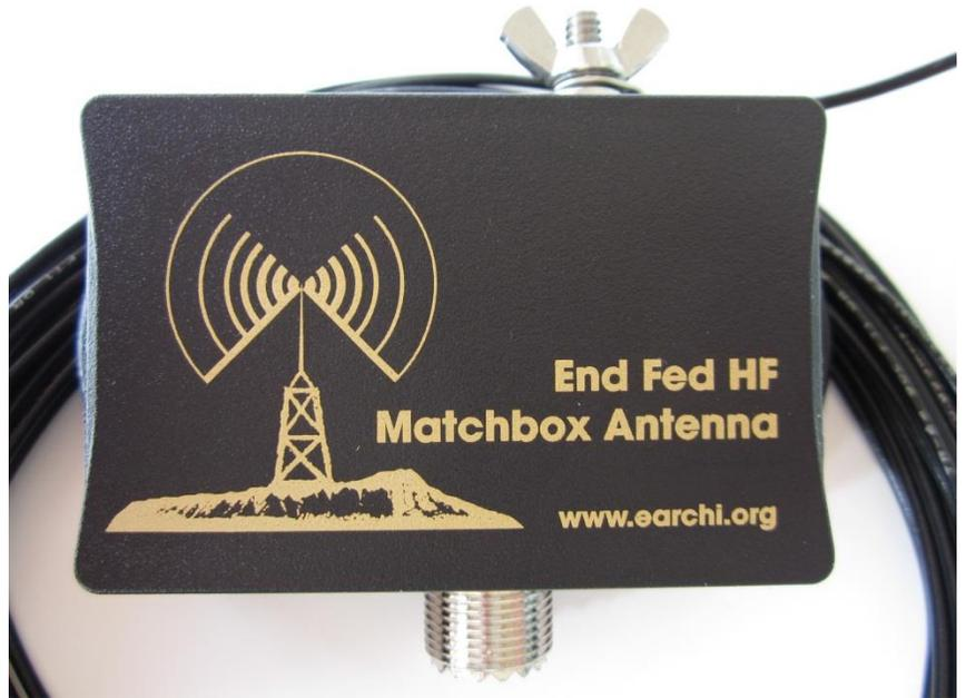
Some tuners, in particular internal tuners, may not tune the full 80-6 meter range. You may need to try different wire lengths to optimize your antenna configuration. If you are having difficulty getting your rig to tune, start with a 26' wire. This should produce good results on at least 40-6 meters using the narrowest performance range of internal tuners. Best performance is achieved with a coax of 16' or longer.
