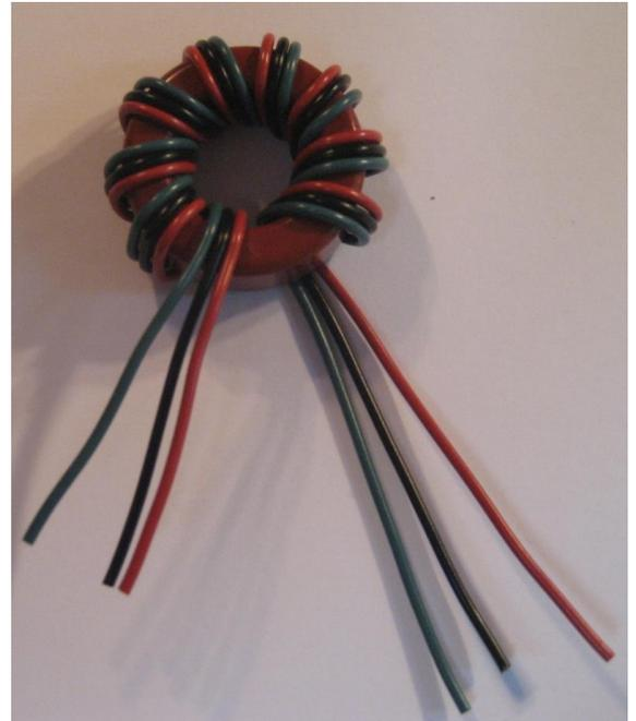
Next, trim, crimp together and solder **the left black wire** with the **right red wire**. When the step is completed, it will look like the photo on the right:
